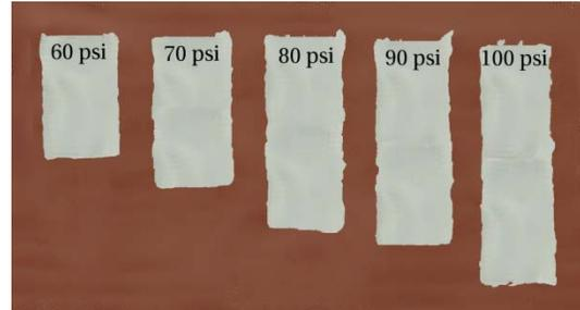
The image above shows an area blasted with different nozzle pressures. Each section was blasted for 5 minutes. This demonstrates how important it is to maintain correct nozzle pressure in order to increase production and decrease abrasive waste. Blasting at 60 psig for 5 minutes cleaned 5 ft<sup>2</sup> whereas blasting at 100 psig for 5 minutes cleaned 10 ft<sup>2</sup>. "Twice the area in the same amount of blast time."
