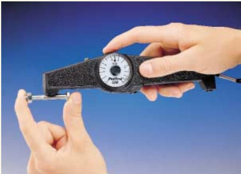
***For the non-destructive measurement of non-magnetic coatings such as (paint, enamel, plastic, galvanizing, metalizing, plating, etc.) on STEEL.***
