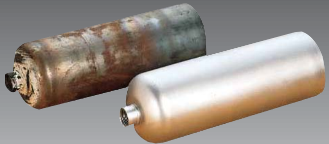
Cylinder surface profiled with aluminum oxide
