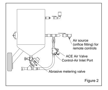
**2.5** Refer to the remote control system manual for which the valve is used, as additional set up may be required.
