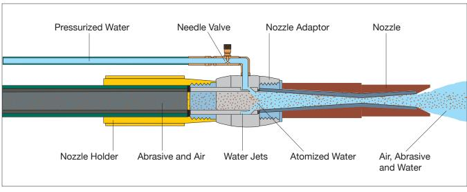
The Wetblast Injector is an economical kit that adds wet-blasting capability to most conventional dry-blast machines.
