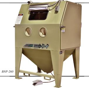
ZERO BNP Wetblast cabinets deliver affordable, dust-free media blasting to efficiently clean and finish all kinds of parts. The wetblast process produces a smooth surface, a bright shine, and does not produce static electricity common in dry blast operations.
