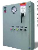
or booths with automatic air balancing systems. Each control panel is designed for a single point wiring connection. All control wires are numbered for easy wire identification. All components are labeled to match electrical schematic. Includes terminal strip for field wiring.
